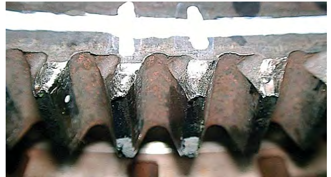
Examples of worn ring gear teeth.
